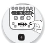
2- Then adjust the setting(s) using the +/- selector (B6). For safety reasons, it is not possible to set a temperature without setting a cooking time.
